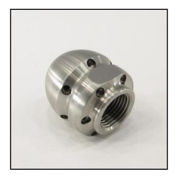
The Multispray Nozzle is especially good in bends and long straights. With its 6 30 degree spray angles, grease and sand gets jetted far back in the pipes. Also comes with front spray for removal of blockades.
